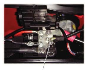
Slave start connector in the plenum chamber
